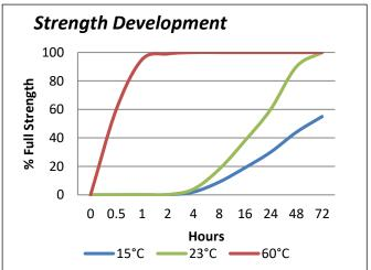
Graph shows typical strength development of bonded components. An increase of 8°C in temperature will halve the cure time. Lower temperatures will result in a slower cure time.
