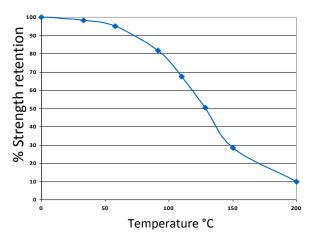
4UV80 can withstand higher temperatures for brief periods (such as for paint baking and wave soldering processes) providing the joint is not unduly stressed. The minimum temperature the cured adhesive can be exposed to is -55°C (-67°F) depending on the materials being bonded.
