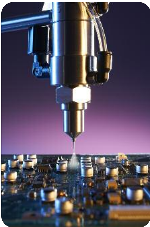
TS5540-MS - spraying conformal coating.
